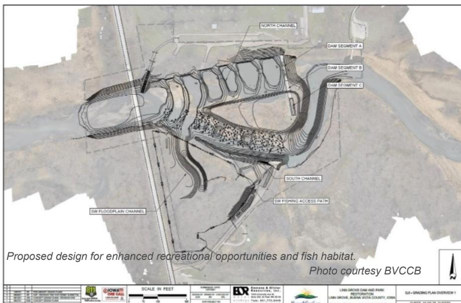
flood events. An existing floodplain slough southwest of the dam site will also be restored. The two channels will be designed to safely accommodate fish passage, fishing access, and passage of paddlecraft during normal flow. The overall design returns the river to a more ecologically sound, sustainable, and safe public amenity.
